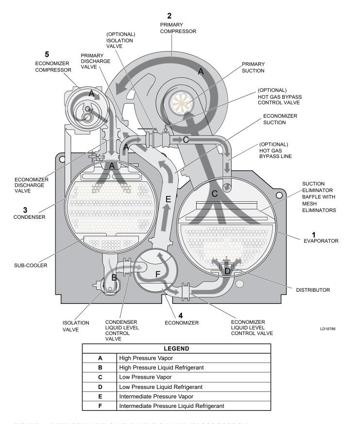
FIGURE 7 - REFRIGERANT FLOW THRU THE CHILLER (CROSS SECTION)
