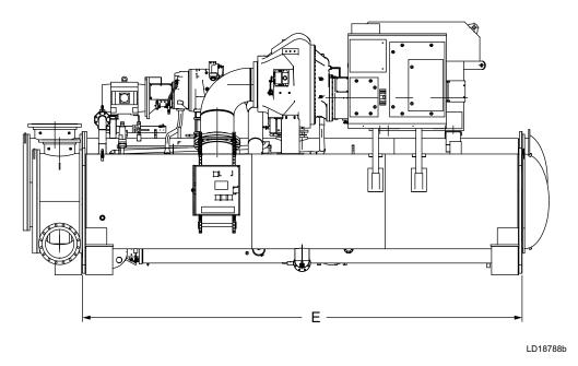
FIGURE 19 - YK-EP STYLE B FRONT VIEW DIMENSIONS
