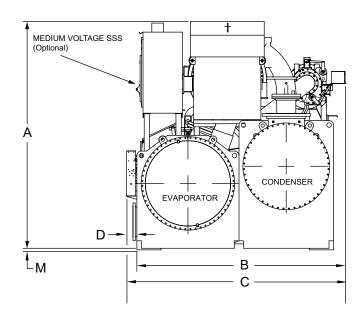
FIGURE 18 - YK-EP STYLE B SIDE VIEW DIMENSIONS
