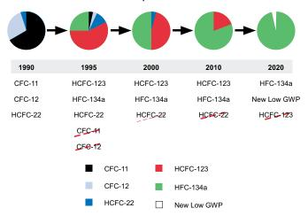
FIGURE 1 - USE OF HFC-134A IN CENTRIFUGAL CHILLERS
