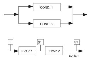
FIGURE 16 - SERIES EVAPORATORS PARALLEL CONDENSERS
