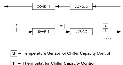
FIGURE 17 - SERIES EVAPORATORS SERIES-COUNTER FLOW CONDENSERS
